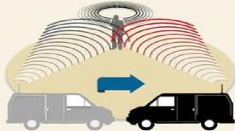
4. The vehicle can then move to another location and again measure the phone's signal strength.
