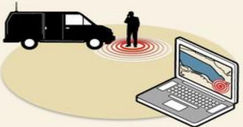
5. By collecting signal strength in several locations, the system can triangulate and map a phone's location.
