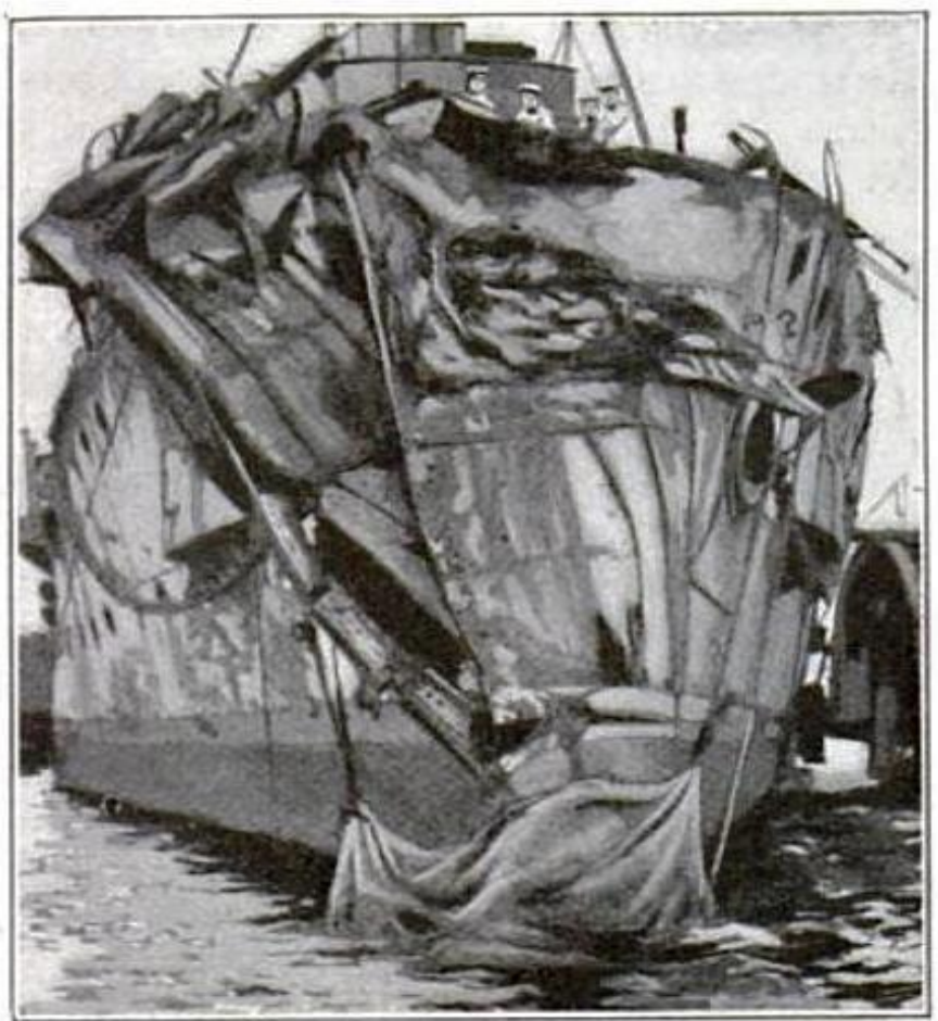
The Bow of the "Hawke," the Damage being so Great That the Ram Has Been Mashed Flat
